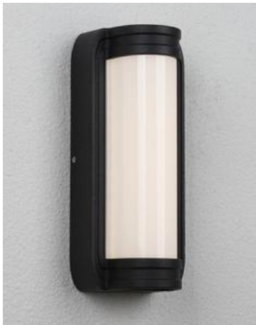
ITEM NO: CY262 POWER: LED 12W CCT: 3000K/4000K/6000K Voltage: AC 85-265V 50/60HZ Size: 280*120*90mm
